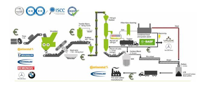
This diagram presents an example of how one tonne of tyres is processed. In order to guarantee the product safety and quality of its end products, Pyrum operates its own tyre shredder. The volume flow and the quality of the input materials can thus be managed and monitored in a targeted manner.
