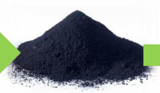
Milled rCB 10 - 14 µm
