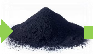
Milled rCB 10 - 14 µm
